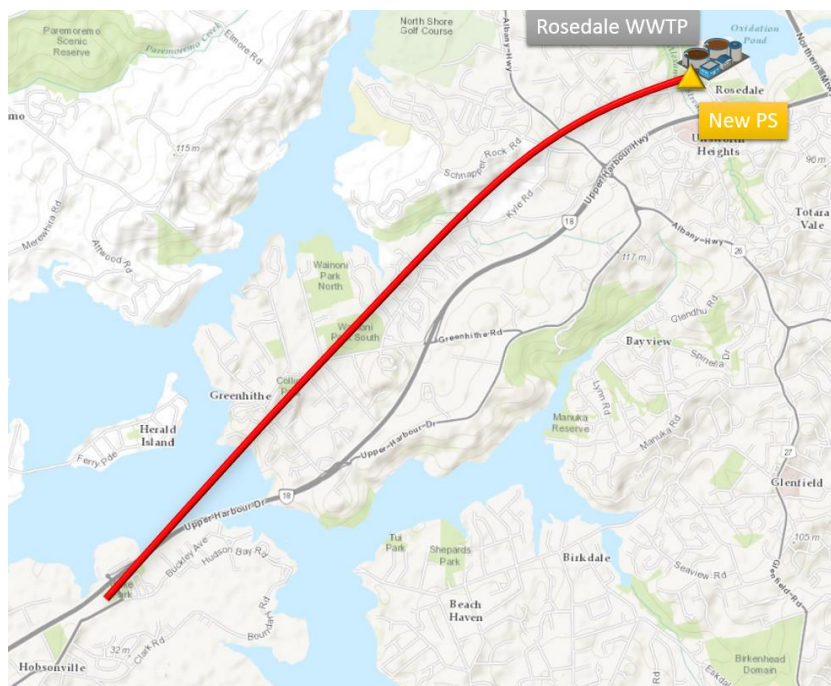
Figure 4-9: Option 7 – Deep Tunnel – Western Alignment
