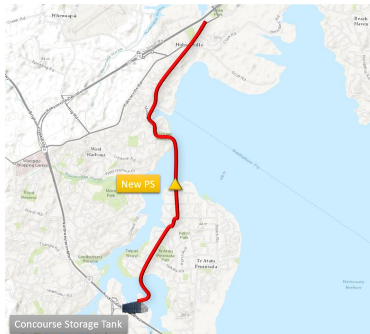
Figure 5-8: Option 6 – Matipo Road – Alternative Pipeline Alignment
